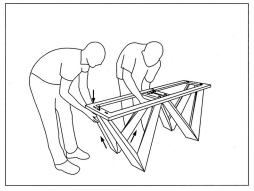
Install the last leg with the frame. Match the number on the leg and frame to place leg on the right position.
