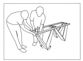
Install the third leg with the frame. Match the number on the leg and frame to place leg on the right position.
