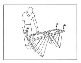
Install dowel "B" into the hole on all four corner.
