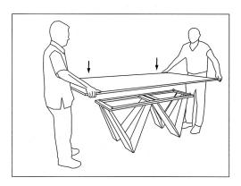
Place the top on frame, follow the dowel to guide the position.
