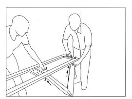
Install first leg with the frame. Match the number on the leg and frame to place leg on the right position.
