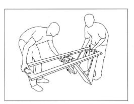
Install the second leg with the frame. Match the number on the leg and frame to place leg on the right position.
